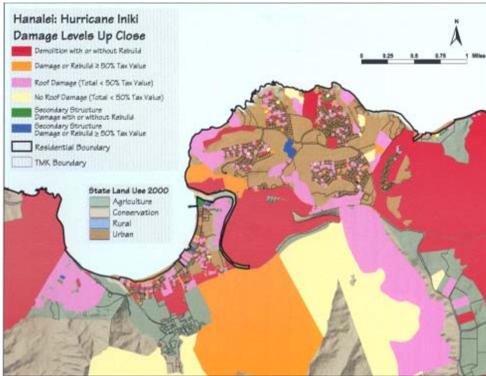
*Figure 4 – A Detailed Wind Damage State Map by Property Parcel for Hanalei and Princeville*
